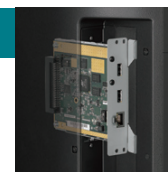
An optional board can slide into the slot on the back of the monitor.
